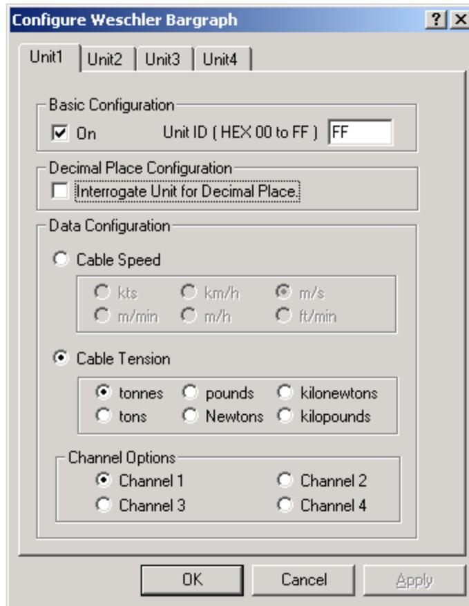
This device can be configured to receive data from up to four inputs from the Weschler unit. Each input is configured individually from the four available tabs. To select and configure each input, select (check) the On option and enter the Unit ID. The ID is in HEX code 0X00 to 0XFF, though only the last 2 characters are entered. These characters can also be numbers depending on the setup of the system.
